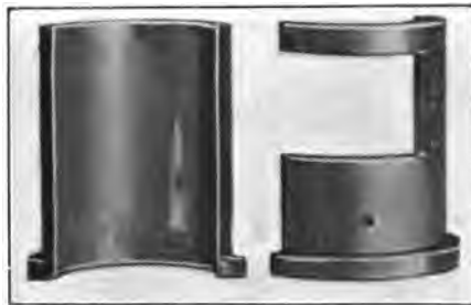
FIG. 157.—A difficult bearing to broach.
